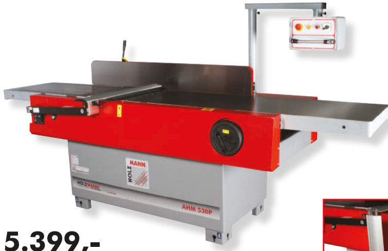
klappbare CPS Hobelwellenabdeckung CPS cutter block protection
