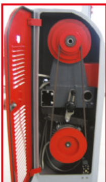
stabiler Riemenantrieb solid and smooth belt run
