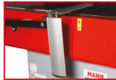
klappbare CPS Hobelwellenabdeckung CPS cutter block protection
